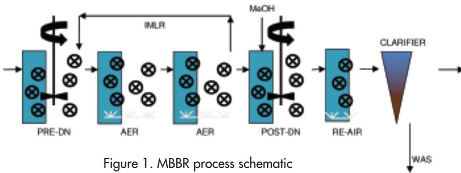
Figure 1. MBBR process schematic
