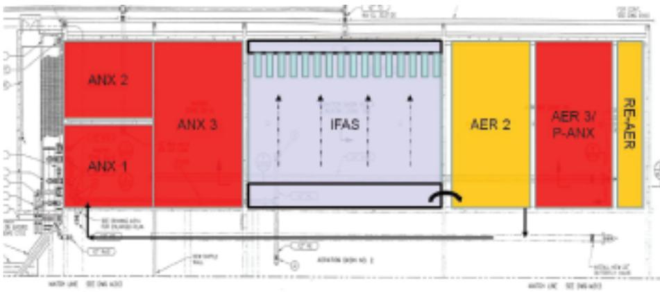
Figure 10. Redirect flow perpendicular to original basin flow scheme
