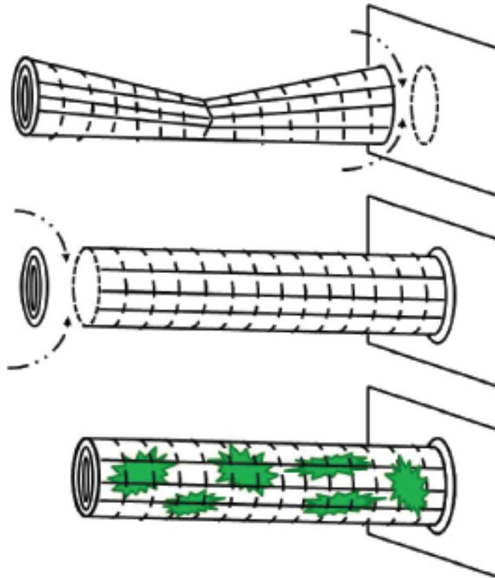
Figure 9. Modes of cylindrical screen failure: structural collapse (top), inadequate end cap installation (middle), and plastic biofilm carrier or trash accumulation (bottom)
