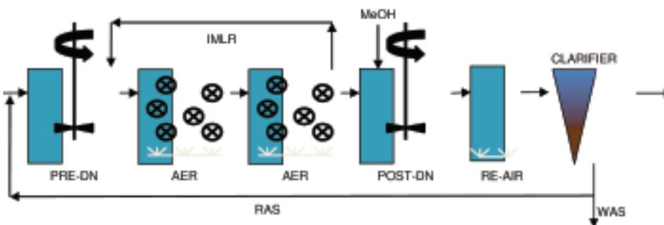
Figure 2. IFAS process schematic
