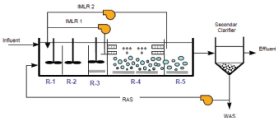
Figure 12. Split IMLR flow using a series of internal recirculation pumps
