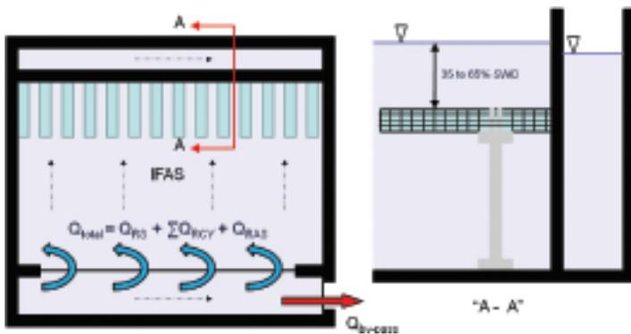
Figure 11. Wet-weather bypass around the IFAS zone
