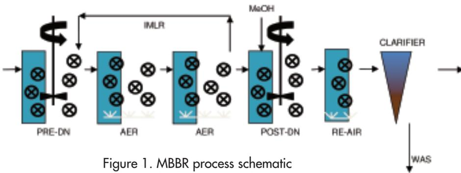
Figure 1. MBBR process schematic
