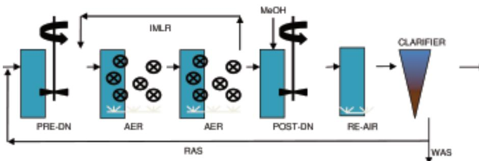
Figure 2. IFAS process schematic
